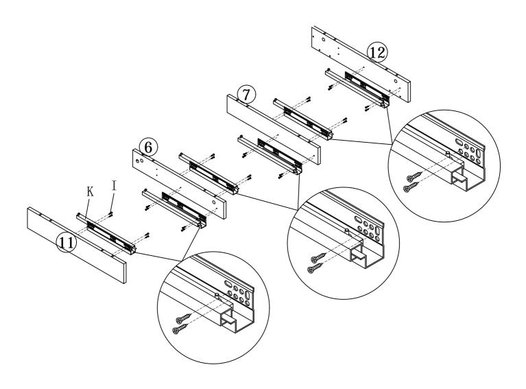
Use wood screw I and philips head screw driver to attach drawer slides K to end panel and partition 11&12&6&7.
