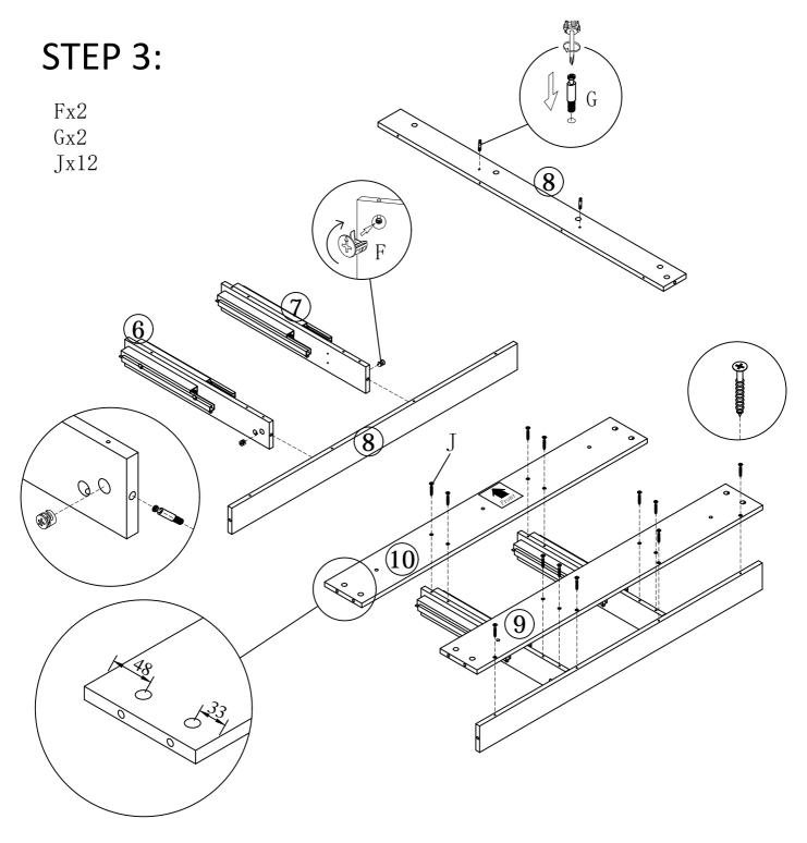
Turn the center partition 6&7 upside down,use philips head screw driver to fasten bolt F on inserts of back panel 8, bottom panel 9&10, then insert the bolts G on back panel 8 through end holes of center partition 6&7, put on cam unit F and fasten to secure. Use philips head screw driver and wood screw J to attach bottom panel 9&10 to bottom edge of center partition 6&7.
