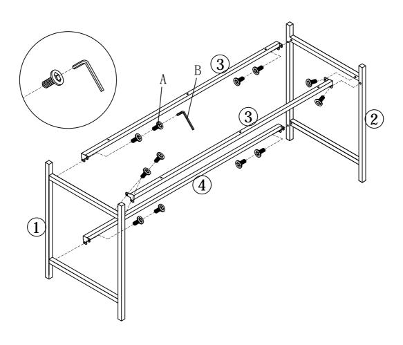
Use bolt A and allen Key B to connect stretchers 3 and 4 with side frames 1&2. Make sure all parts sets leveled then fasten all bolts to secure.
