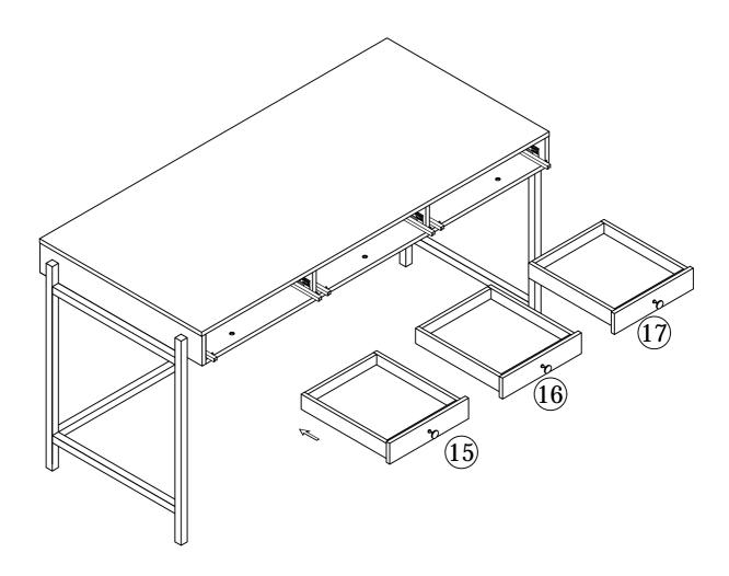
Pull out the drawer slides and carefully align the pin on drawer slides with the hole on drawer box then fix the clip to secure the drawer. Whenever drawer adjustment of drawers needed, please spin the pin on drawer slides to set it level.
