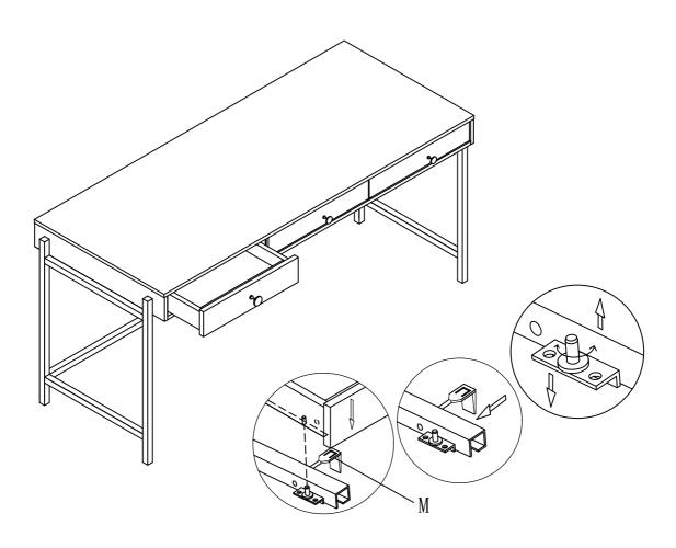
Switch the button with hand to slightly adjust the height of drawer sides in order to sent the drawer leveled. Insert the plastic clip M through the slide to the hole on drawer sides.
