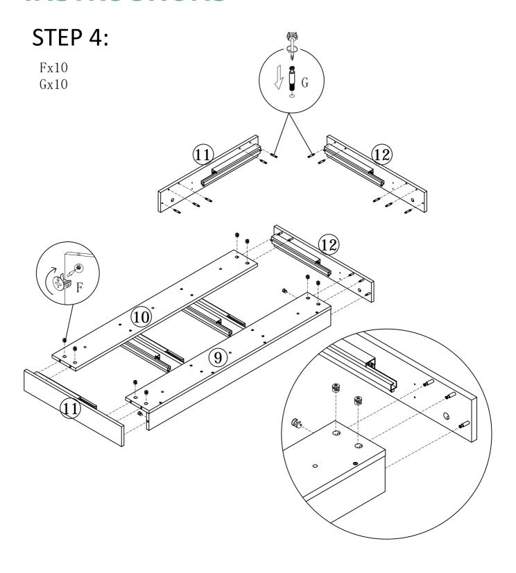
Use philips head screw driver to fasten bolt G on inserts of end panel 11 & 12, back panel 8, then insert the bolts G on end panel 11 & 12 through end holes of bottom panel 9 & 10, put on cam unit F and fasten to secure.
