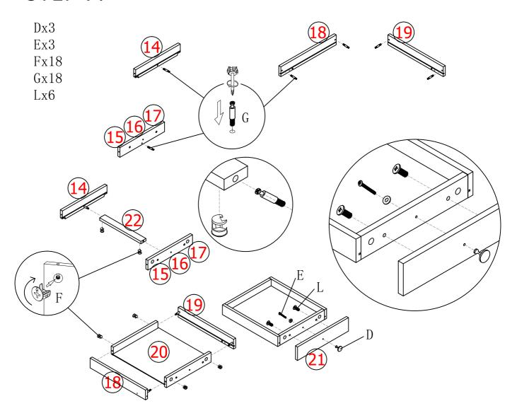
Use philips head screw driver to fasten bolt G on inserts of drawer front 15/16/17 and back 14 , put on cam unit F and fasten to secure.
