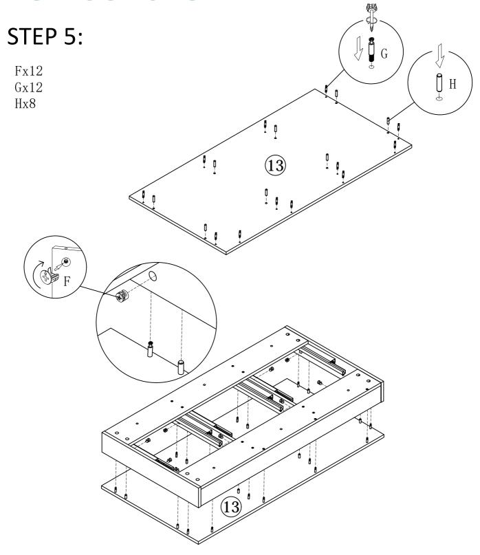
Use philips head screw driver to fasten bolt G on inserts of table top 13, Insert all dowels H to holes on back side of table top 13 then insert the bolts G on table top 13 through end holes of end/back/bottom panels assembly (6&7&8&9&10&11&12), put on cam unit F and fasten to secure.
