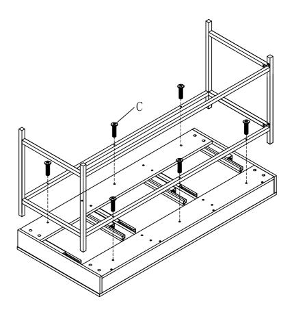
Use philips head screw driver and bolt C to attach the metal frame assembly to bottom of upper unit, make sure all edges align then fasten to secure.
